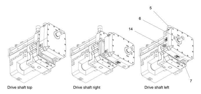
Fig. 2: View of the SiloKing type LS with adapter gear
