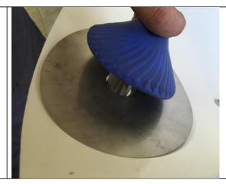
At the same time the person on the outside places the manifold, gasket, t-handle gasket and t-handle over the protruding stem.
