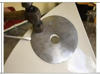
Examples of badly worn wear plates. Under normal working conditions, wear plates should not be allowed to get this bad, as the wear can extend to the cone itself.
