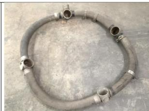
Once the exterior assembly has been removed, the person on the inside of the tanker can remove the old aerators and stems.
