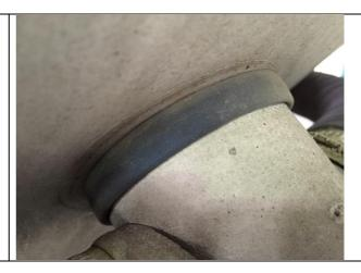
The whole assembly (including the 1.5" hose) should now be removed. Check the hose carefully for any cracks, and ensure clamps are tight around the manifolds (without overtightening).
