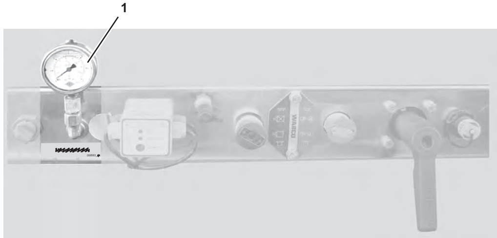
Illustration 4.9 Axle load indicator (bellows pressure)
