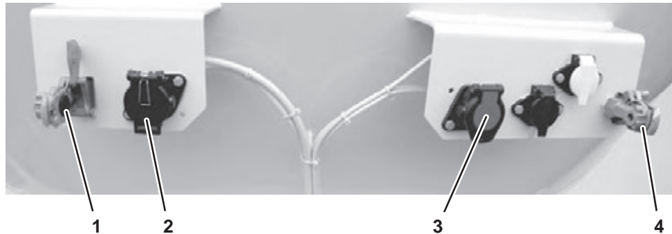
Illustration 4.2 Compressed air brake system couplings
